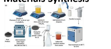
Figure 1 Schematic representation of the synthesis procedure of MVO powders
