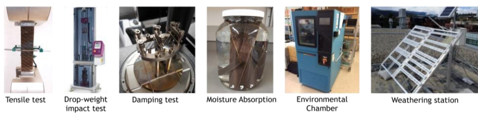
Figure 1: Methodology summary for biocomposite mechanical characterization under accelerated and natural ageing conditions.
